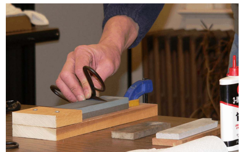
A self-made “cradle” to support and stabilize the stone
